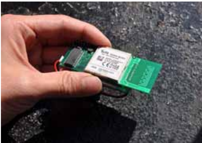
> Figure 11: The custom-designed electronic tag for the Trash Track Project. SENSEable City Lab ©
