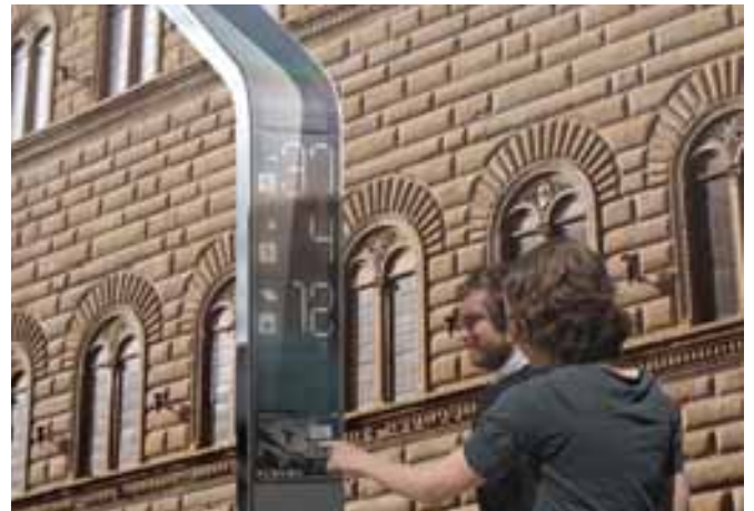
> Figure 7: Rendered view of a possible implementation of EyeStop as an information pole with interactive touch screens and E-ink digital displays. SENSEable City Lab ©
